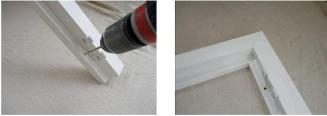
The standard Z frames do not have any pre-drilled frame holes.
