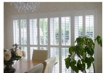
Z frame Tposts are not supplied with removable inserts, they are only fixed via the top and bottom frames.
